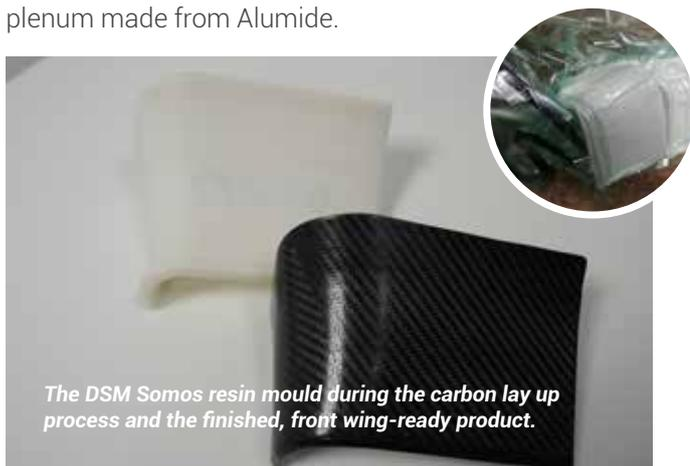
*The DSM Somos resin mould during the carbon lay up process and the finished, front wing-ready product.*
